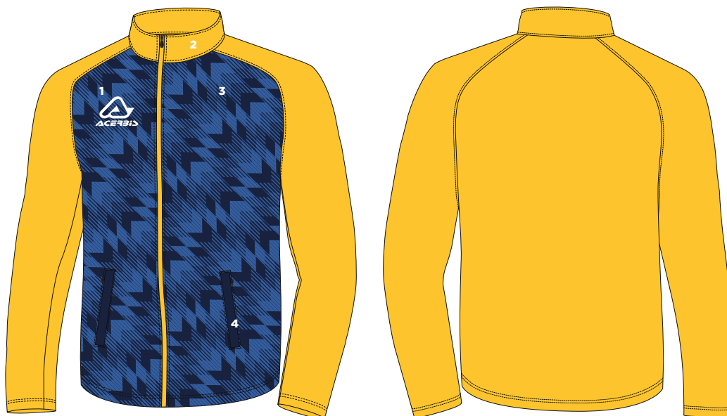
1 Heat transfer logo - 2 Inner neck heat transfer - 3 Sublimation - 4 Zipped welt pockets
